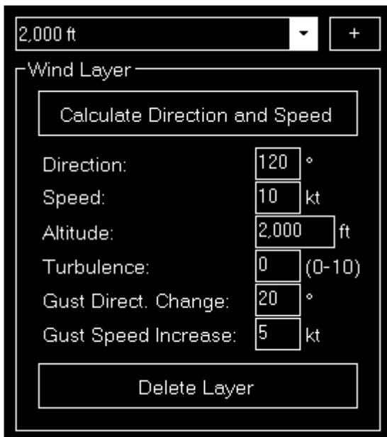
The screenshot shows a dialog box titled "Wind Layer" with a dropdown menu at the top set to "2,000 ft" and a "+" button. Below the title bar is a "Calculate Direction and Speed" button. The main area contains six input fields: "Direction" (120 °), "Speed" (10 kt), "Altitude" (2,000 ft), "Turbulence" (0 (0-10)), "Gust Direct. Change" (20 °), and "Gust Speed Increase" (5 kt). At the bottom is a "Delete Layer" button.
