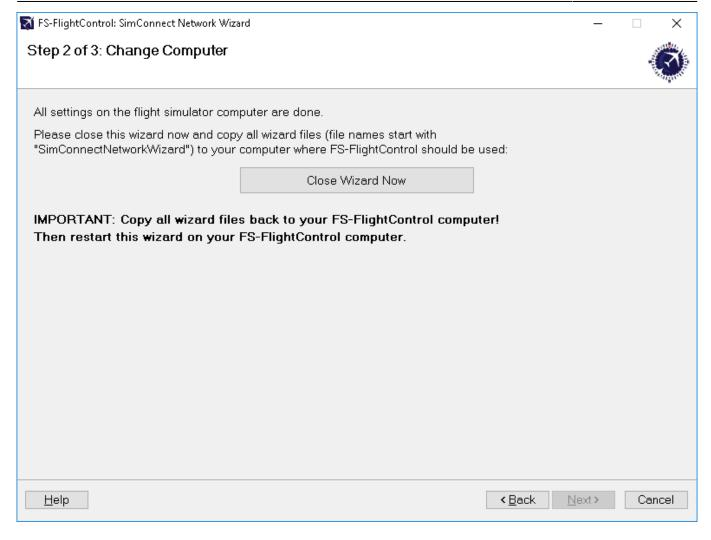
Now everything is done on the flight simulator computer and therefore it is time to go on with the computer that should run FS-FlightControl.
