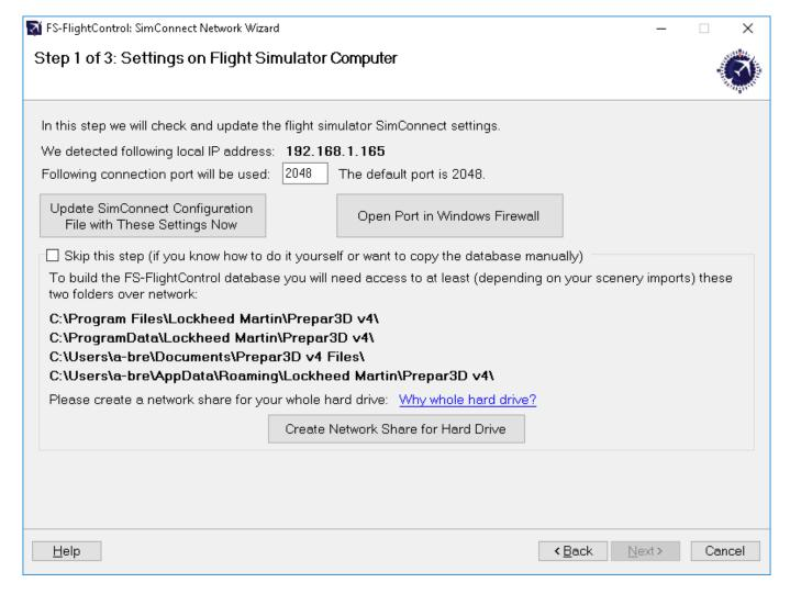
On the next screen, the first step in the setup process, all settings on the flight simulator computer are done.
