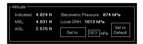
In the altitude section the current aircraft altitude above mean sea level (MSL) as well as the altitude above ground level (AGL) is displayed.
