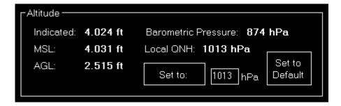
In the altitude section the current aircraft altitude above mean sea level (MSL) as well as the altitude above ground level (AGL) is displayed.
