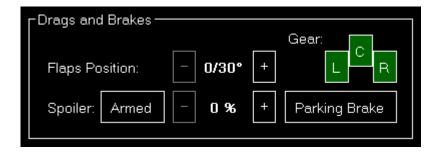
Use this section to see and change the current flaps, gear, spoiler and parking brake status.
