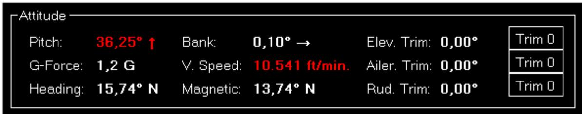
Here the current aircraft pitch and bank angle, the G-force, vertical speed, heading and elevator trim is displayed. You can also trim the elevator back to zero with just one click on the button.
