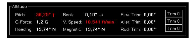
Here the current aircraft pitch and bank angle, the G-force, vertical speed, heading and elevator trim is displayed. You can also trim the elevator back to zero with just one click on the button.
