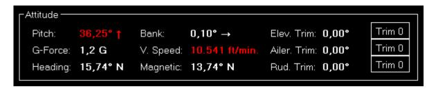
Here the current aircraft pitch and bank angle, the G-force, vertical speed, heading and elevator trim is displayed.
