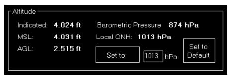
In the altitude section the current indicated altitude, the altitude above mean sea level (MSL) as well as the altitude above ground level (AGL) is displayed.
