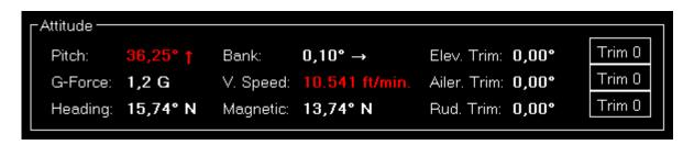
Here the current aircraft pitch and bank angle, the G-force, vertical speed, heading and elevator trim is displayed.
