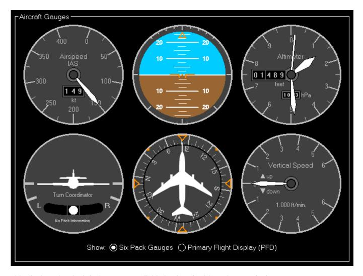
This displays the six default gauges available in aircraft with analogue avionics.
