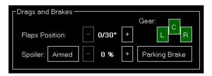
Use this section to see and change the current flaps, gear, spoiler and parking brake status.
