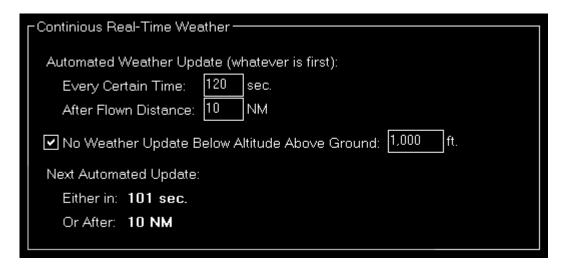
To enable continues real-time weather just activate the corresponding check box. This will enable automated real-time weather updates for all weather stations around the current aircraft location.
