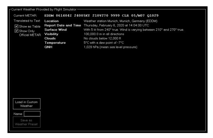
In this section the current weather is displayed as METAR code and translated text.
