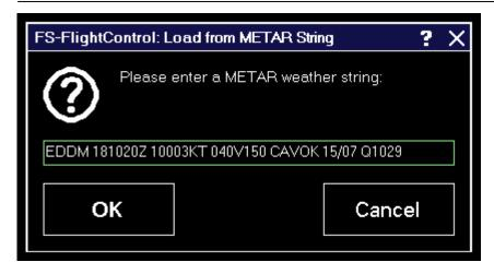
If you have a METAR string as starting point for your custom weather enter it here. This will decode the weather situation defined in the METAR string into the custom weather sections.
