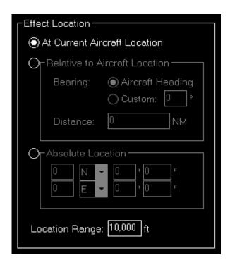
Select here if the effect should be placed at the current aircraft location, relative to the aircraft location or at a custom absolute location.
