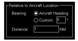
If the effect should be placed relative to the aircraft location, you first need to choose if it should be place in the direction of the current aircraft bearing or in a custom direction.
