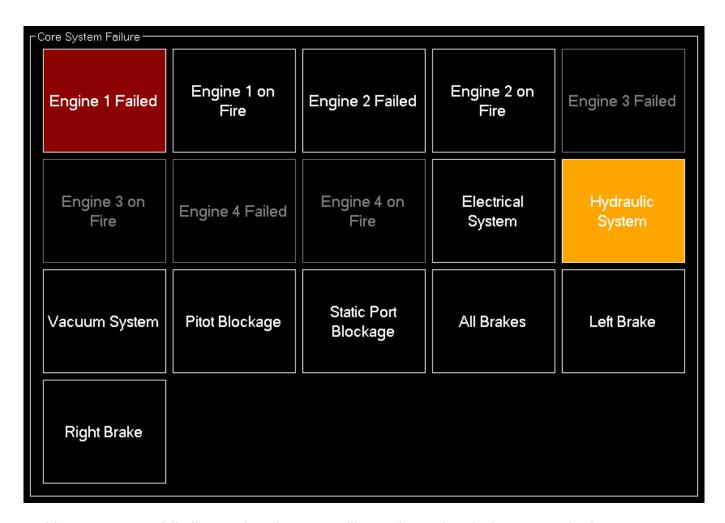
In this area you can fail all core aircraft systems like engines, electrical system or brakes.
