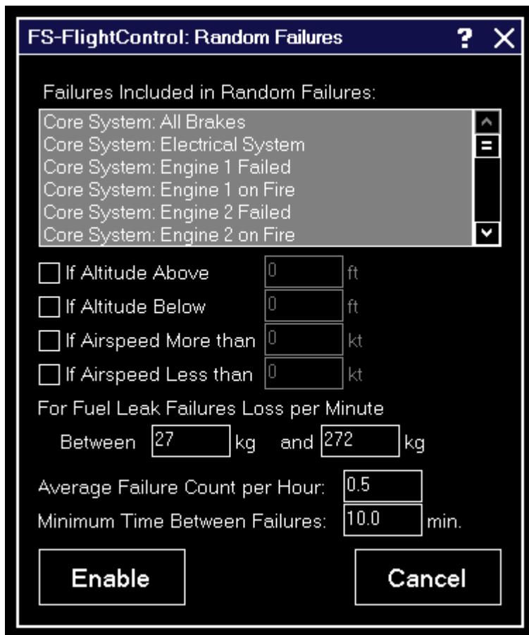
Beside triggering specific failures directly there is also an option to let FS-FlightControl generate random failures.
