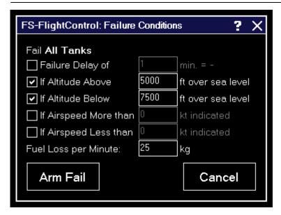
After clicking on a failure button in one of the sections above, these failure condition options will be displayed. Enable the check box before a condition to enable it.
