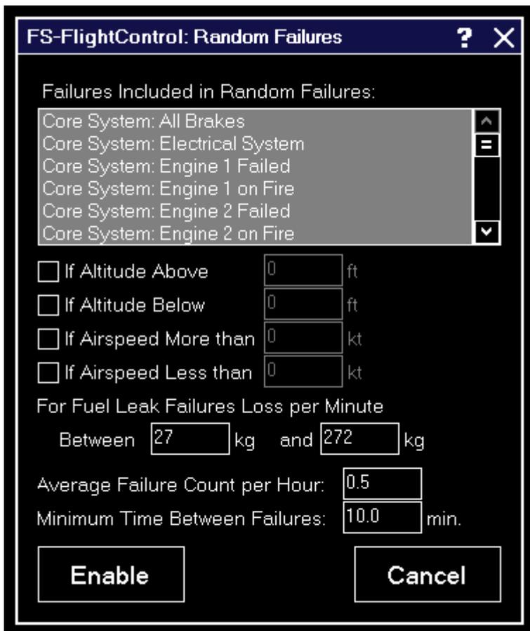
Beside triggering specific failures directly there is also an option to let FS-FlightControl generate random failures.
