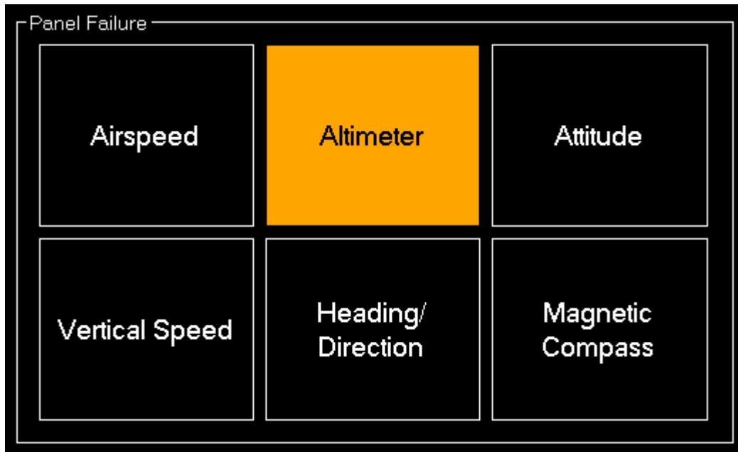
Fail one or more panels here to force the pilot to get along with the situation also without that specific panel systems.
