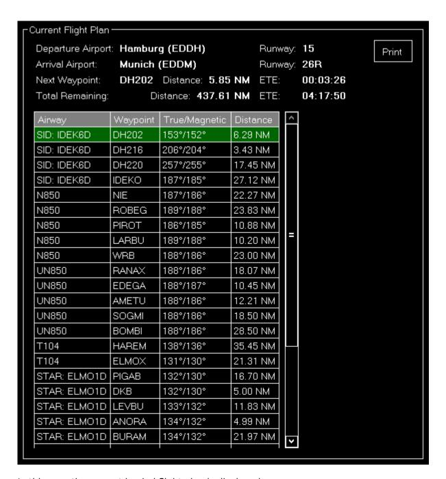
In this area the current loaded flight plan is displayed.
