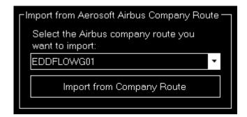
If you have installed an Wilco/FeelThere Airbus product you can also import the Wilco Airbus company route as flight plan.
