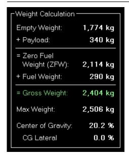
In the weight calculation section the current aircraft weight is calculated in real-time considering the aircraft empty weight, the current payload as well as the remaining fuel in all tanks.
