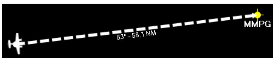
If the start or end point is a moving object (like the user or AI aircraft) the measure arrow will move together with the objects and update accordingly. Additionally, it will show the time en-route based on the ground speed of the first object.
