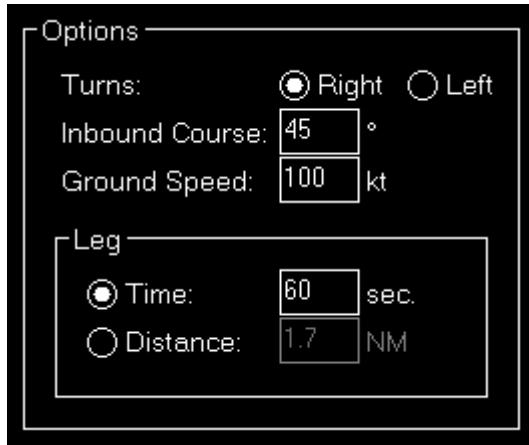
The holding can be a right (standard) or left (non-standard) holding.
