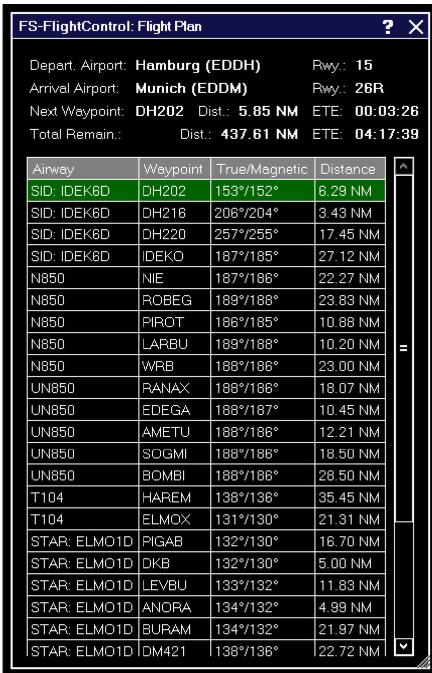
This dialog is displayed as long as the flight plan mode is enabled. The displayed flight plan tables has the same functionality as on the **Flight Plan** module.
