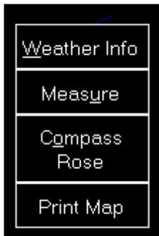
Weather Info toggles the display of a wind arrow in the top center of the map. In partly active state only the wind arrow itself is displayed and in full active state additionally the current wind speed and true direction separated with a T as well as the visibility range and temperature are displayed.
