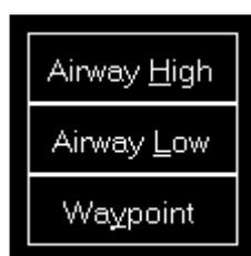
**Airway High** toggles the display of high (jet) airways together with their connecting waypoints. In partly active state only the airways and waypoints themselves are displayed and in full active state additionally the airway names and waypoint idents.
