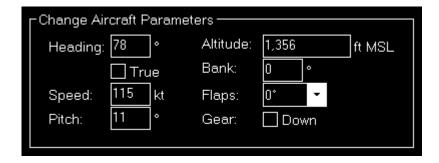
All other aircraft parameters like heading, altitude, speed, pitch and bank angle are pre-filled with the current aircraft values.
