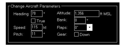
All other aircraft parameters like heading, altitude, speed, pitch and bank angle are pre-filled with the current aircraft values.
