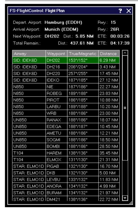
This dialog is displayed as long as the flight plan mode is enabled. The displayed flight plan tables has the same functionality as on the *Flight Plan* module.
