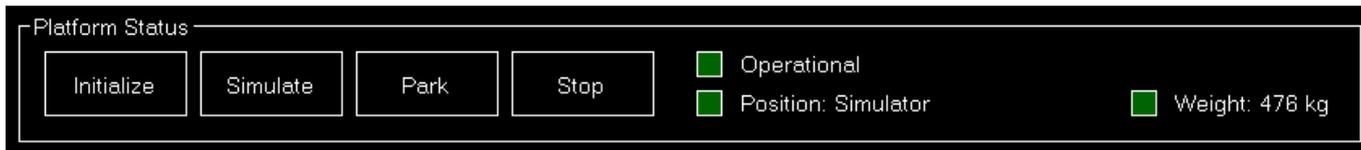
The platform status shows if it is currently operational as well as what the current position and weight of the platform is.
