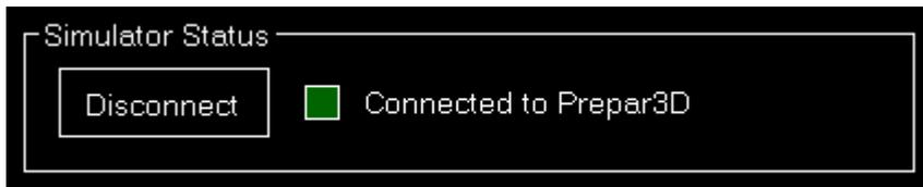
The simulator status shows if CLS2Sim is currently connected to a flight simulator. This also includes the name of the flight simulator.
