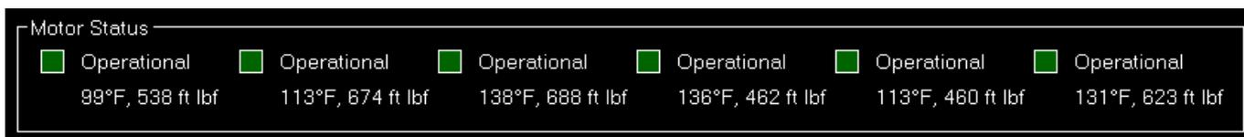
The motor status shows if each of the motors is currently operational as well as what the current temperature and force is.
