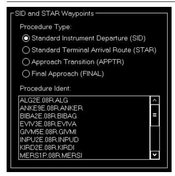
You can place your aircraft directly on a waypoint of a Standard Instrument Departure (SID) or Standard Terminal Arrival Route (STAR).
