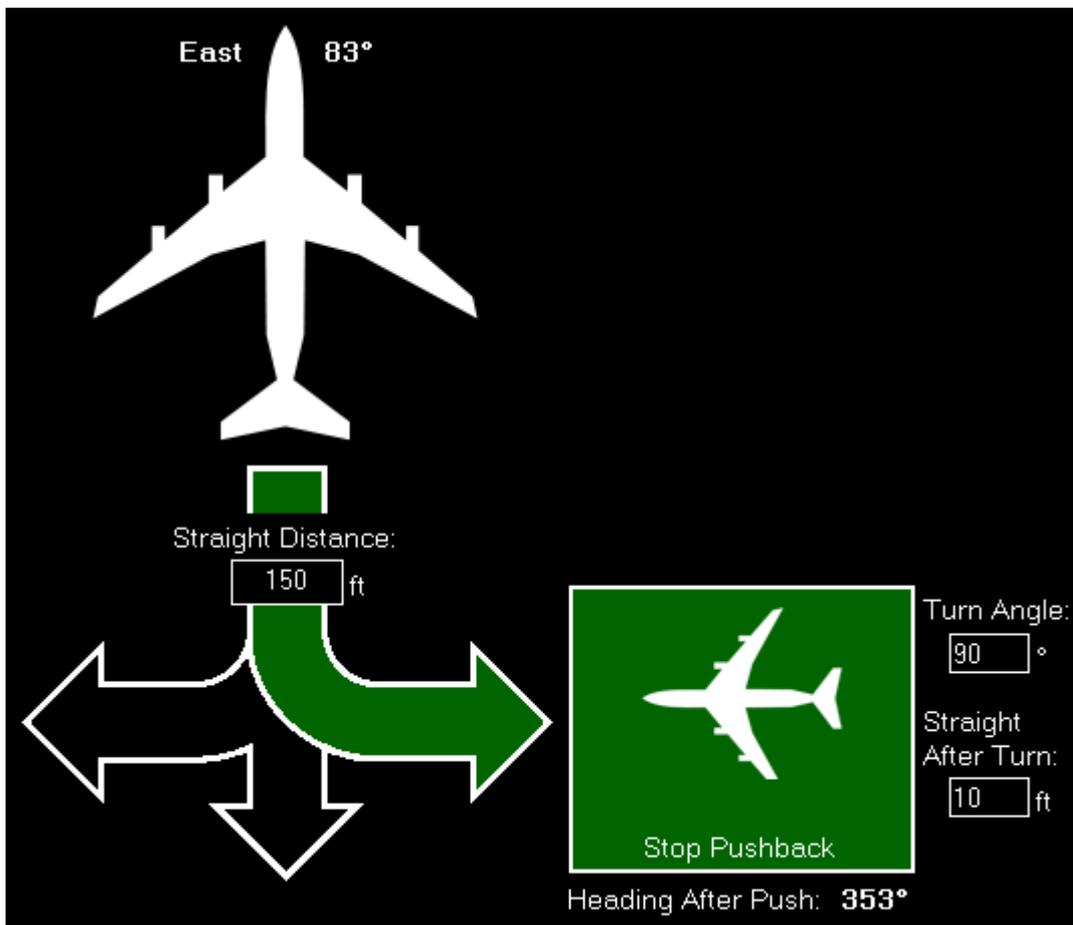
The pushback operation will stop automatically after the defined push distance and in case of pushback to left or right the turn including the additional straight distance after turn has been reached.
