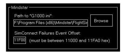
You can enter the path to the Mindstar G1000.ini file here. The Mindstar connection then can be used in the *Failures* module.
