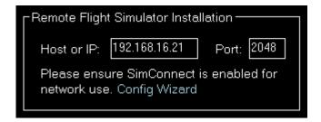
If you want FS-FlightControl to access a flight simulator installation that is not located on the same computer as FS-FlightControl itself, these SimConnect Network Access parameters need to be defined.
