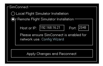
You can choose here if FS-FlightControl should connect to a local or remote flight simulator installation.
