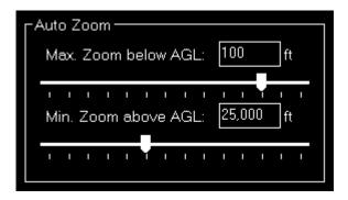
The *Map* module also features an auto zoom function which will zoom the map in and out according to the current aircraft altitude.
