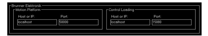
This section allows to configure the motion interface to Brunner Elektronik products.
