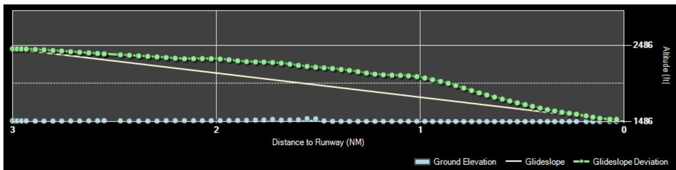
On the lower approach graph the current aircraft altitude above mean sea level (MSL) as well as the ground altitude is shown.
