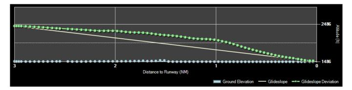
On the lower approach graph the current aircraft altitude above mean sea level (MSL) as well as the ground altitude is shown.
