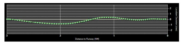
The localizer deviation graph shows the horizontal deviation from the runway localizer (usually the center of the runway) on your approach.
