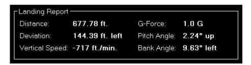
After the approach has been completed and the aircraft is landed, this landing report shows detailed information about how well the landing was.
