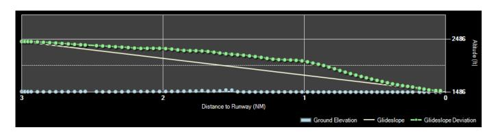
On the lower approach graph the current aircraft altitude above mean sea level (MSL) as well as the ground altitude is shown.
