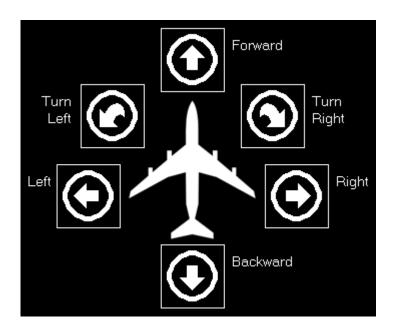
Here you can slew the aircraft forward and backward, left and right as well as turn it left and right.
