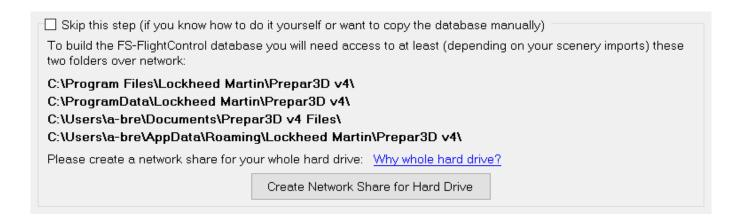
Beside accessing the flight simulator directly via SimConnect, you will also need to build the FS-FlightControl database that contains all the information about airports, navigation aids and so on. To be able to build that FS-FlightControl needs access some flight simulator directories.
