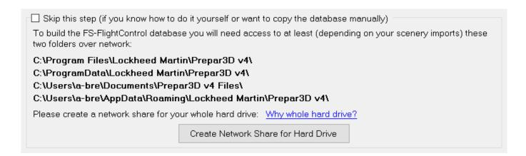
Beside accessing the flight simulator directly via SimConnect, you will also need to build the FS-FlightControl database that contains all the information about airports, navigation aids and so on. To be able to build that FS-FlightControl needs access some flight simulator directories.
