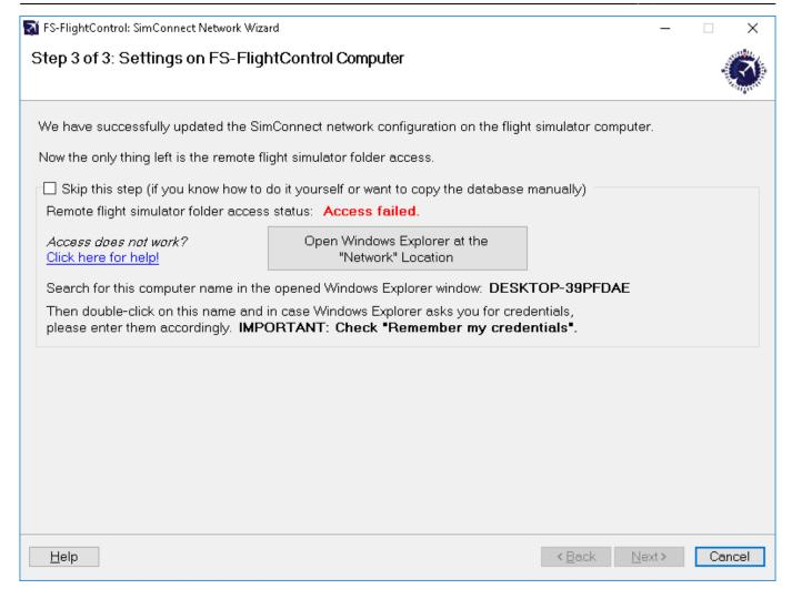
After you have started the wizard on your FS-FlightControl computer you should directly see this screen. Here the configuration on the FS-FlightControl computer will be applied.
