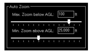
The Moving Map module also features an auto zoom function which will zoom the map in and out according to the current aircraft altitude.
